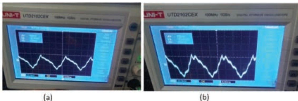
Oscilloscope waveform without fish scale and with fish scale tapping (a) Oscilloscope waveform without fish scale connected (b) Oscilloscope parameters 20mv/division with Time period : 5ms Probe setting 1x Coupling: DC
